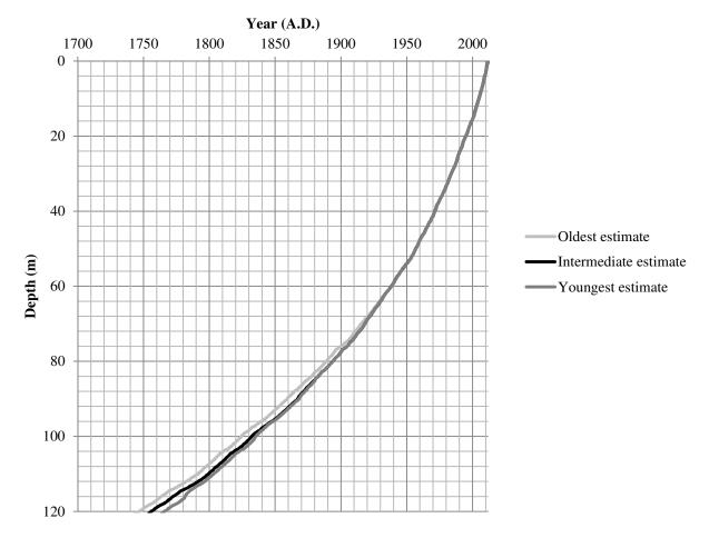
Figure 3. Age-depth relationships reconstructed from the relative dating process. Note that the approach results in no uncertainty above 62.38 m depth (year 1933). At 120 m depth, the uncertainty is  $\pm 10 \text{ years}$ .
