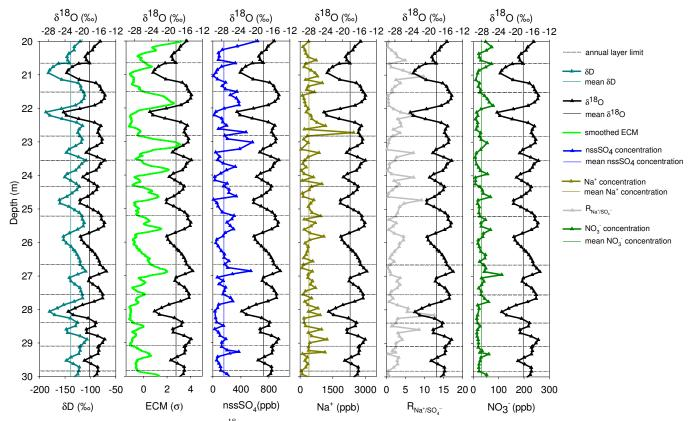
Figure 2. Variations in stable isotopes ( $\delta^{18}O$ ,  $\delta D$ ), smoothed ECM (running mean, 0.1 m), chemical species and their ratios used to constrain annual layer thickness in an example 10 m long section (20 - 30 m depth) of the IC12 ice core. Dashed horizontal lines indicate the annual layer limit (middle of the summer  $\delta^{18}$ O peak).
