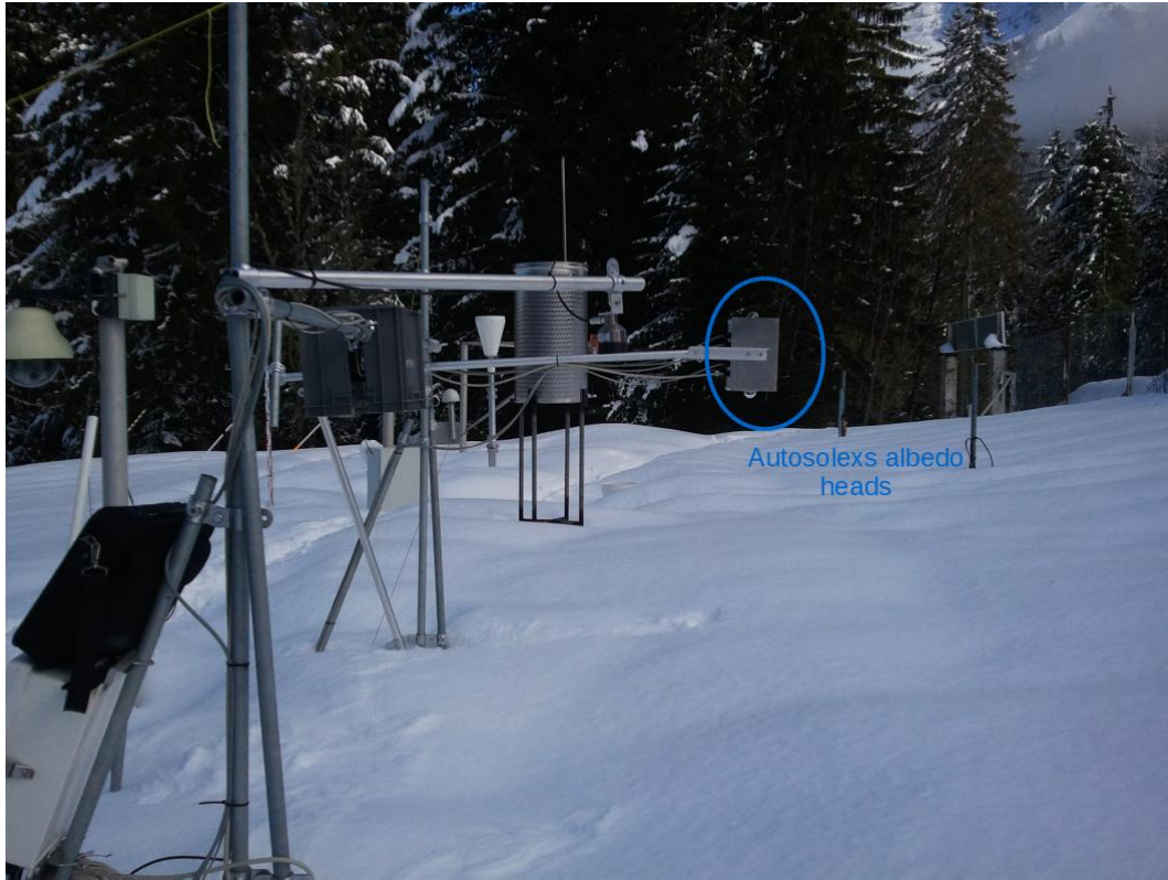
Figure 1. Part of the col de Porte field measurements site on 2014-02-17 14:35. North direction is the left of the picture. The two measurement heads of Autosolexs are circled in blue.
