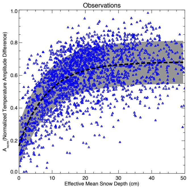
Figure 3: Observed relation between  $A_{norm}$  and effective mean snow depth ( $S_{depth,ef}$ ) along with the resulting exponential fit (dashed line). The grey shading shows the median fit plus/minus the mean scatter ( $O_{err}$ ) of all fits.
