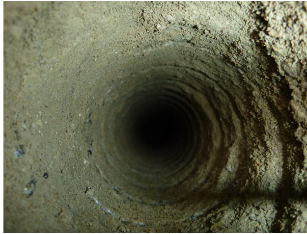
Figure 2. Photo of borehole after completion with gasoline-powered auger. Ice is visible along the walls where the soil was abraded, demonstrating the limited thermal effects of drilling.
