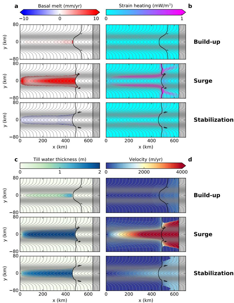
**Figure 4.** Fields of (a) basal melt rate  $m$ , (b) strain heating, (c) till water thickness  $W_{til}$ , and (d) velocity for a representative snapshot for each of the three phases of build-up, surge and stabilization (as denoted by the colored circles in Fig. 3). Thick black contours mark the grounding line and calving front. Bed topography shown by thin gray contours.
