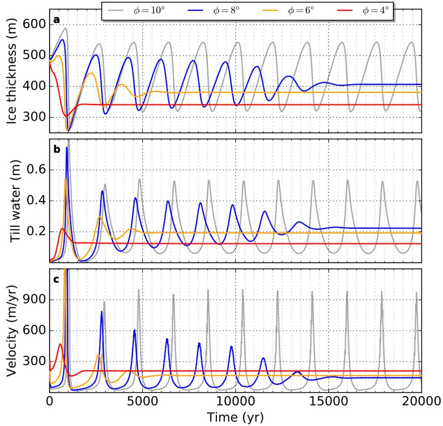
**Figure 6.** Timeseries of (a) ice thickness  $H$ , (b) till water thickness  $W_{til}$ , and (c) ice velocity (all averaged over area of grounded ice) for different values of the till friction angle  $\phi$  ( $\phi \leq 10^\circ$ ). Between  $\phi = 10$  (default case) and  $\phi = 8$  there is a transition from maintained cyclic surging to damped surging.
