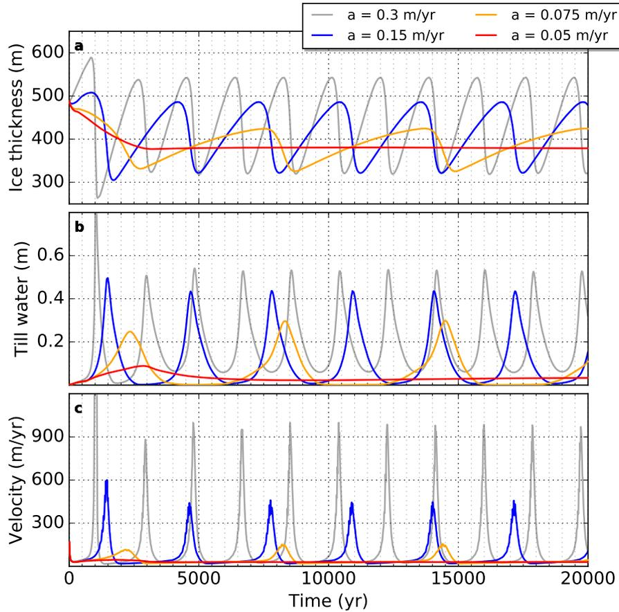
**Figure 9.** Timeseries of (a) ice thickness  $H$ , (b) till water thickness  $W_{til}$ , and (c) ice velocity (all averaged over area of grounded ice) for different values of the surface accumulation  $a$ . With decreasing  $a$  (default case in gray) the surge magnitude decreases and the cycle duration increases such that for sufficiently low accumulation surging is not existent.
