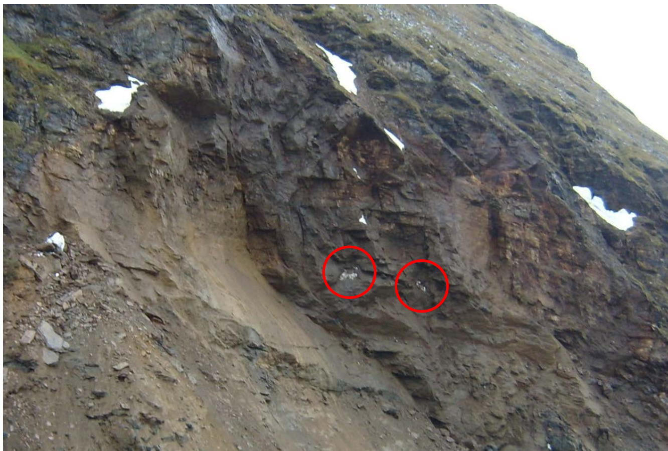
5 Figure 2. Visible in-situ ice (encircled areas) observed in the rockslide failure zone on June 26 th , 2008. The photograph was taken a few hours after the event (Photograph by courtesy of Kjetil Brattlien, NGI).
