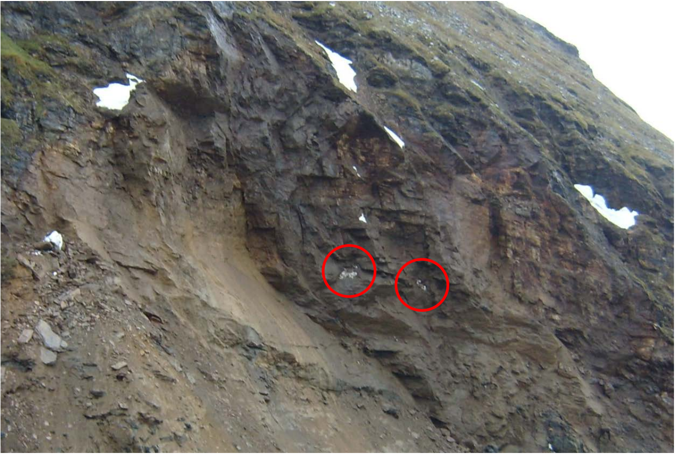
Figure 2. Visible in-situ ice (encircled areas) observed in the rock avalanche failure zone on June 26 th , 2008. The photograph was taken a few hours after the event (Photograph by courtesy of Kjetil Brattlien, NGI).
