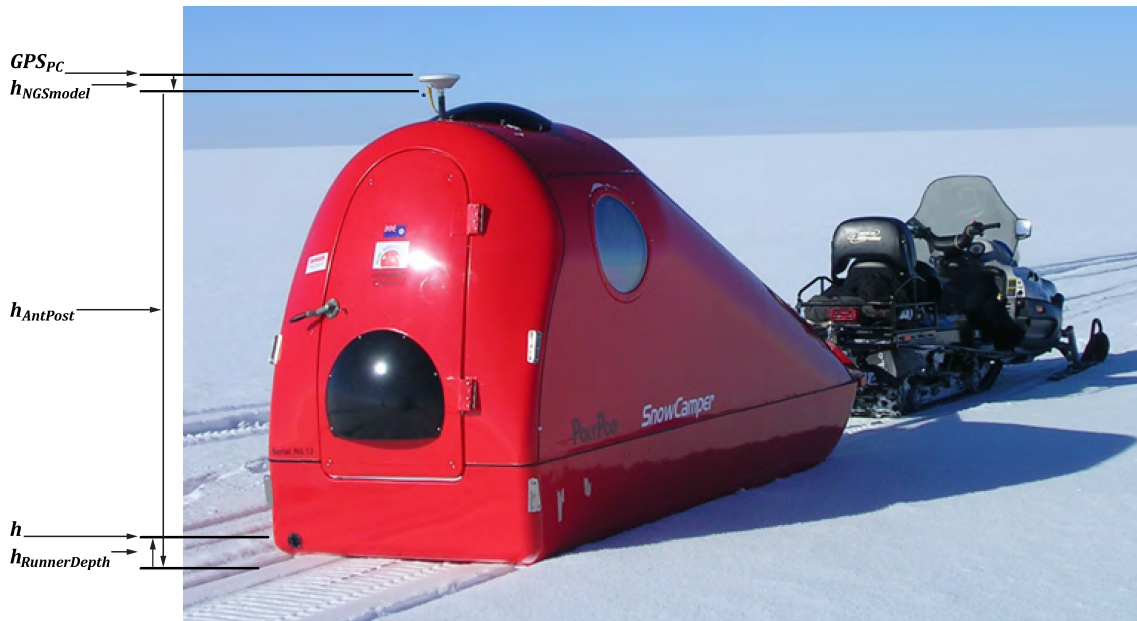
Figure 2: The roving GPS antenna, sled, and snowmobile configuration. GPS_{PC} is the surveyed position solution to the phase center of the antenna, h_{NGSmodel} is the NGS model distance between the antenna phase center and the antenna base plane, h_{AntPost} is the height of the antenna post (Table 1), h_{RunnerDepth} is the depth of the sled runners in the snow surface (Table 1), and h is the snow surface (Equation 1).
