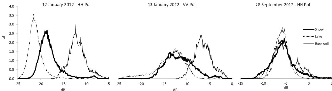
**Figure 8: Radar backscattering of snow, water and soil ground truthing areas for the three selected TerraSAR-X scenes: a. HH-Polarization (12/01/2012), b. VV-Polarization (13/01/2012) and c. HH-Polarization (28/09/2012).**
