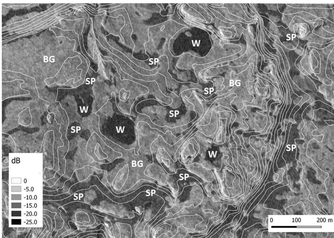
Figure 11: TerraSAR-X SpotLight mode HH polarization backscattering (sigma-nought) scene from 12 January 2012 with examples of visual interpretation of bare ground (BG), water (W) and snow patches (SP). Countour lines at 5 m equidistance.
