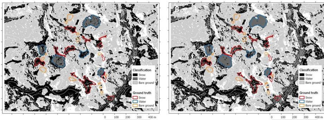
Figure 12: Classification results using: a. backscattering threshold water – wet snow at -20.5 dB, b. backscattering threshold water – wet snow at -19.5 dB.
