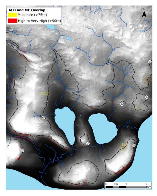
Figure 5: Areas where the ALD and ME maps at CBAWO have overlapping susceptibilities (superimposed over the 1 m shaded relief DEM). The marine limit is denoted by the 60 m contour line.
