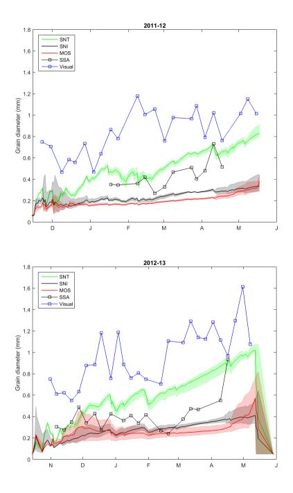
**Figure 4.** Bulk grain diameter evolution for the MOS, SNT and SNI microstructure evolution models and the spread in model results. Observations of bulk diameter were derived from macro-photography (Visual) and from SSA measurements from the IceCube instrument
