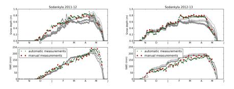
**Figure 3.** Snow depth and water equivalent simulated by the Jules Investigation Model subset used in this study. Grey lines indicate individual JIM subset member simulations. Note that erroneous positive SWE observation points have been removed at the end of the season when snow depth is zero, as this is a sensor artifact related to soil moisture changes.
