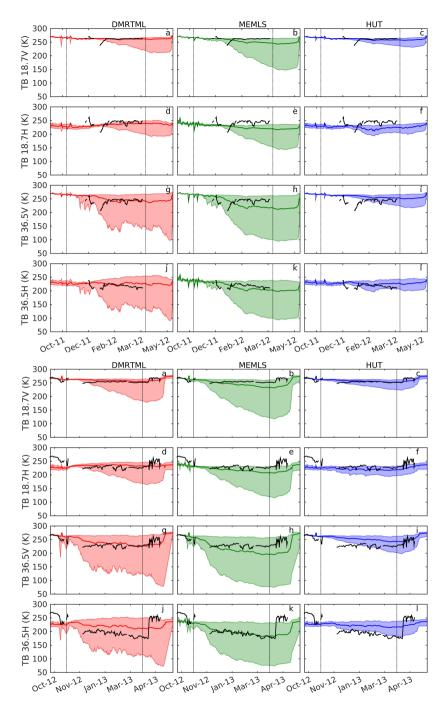
**Figure 5.** Range and mean of brightness temperature over the two winter seasons as simulated with the DMRT-ML, MEMLS and HUT models, driven by 63 JIM outputs and 3 microstructure evolution models. Black lines indicate the observed brightness temperatures. Vertical dashed lines enclose the period of analysis (1st November - 31st March).
