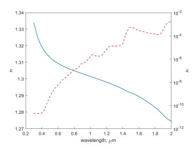
Figure 2. The refractive index of ice after Warren and Brand (2008): real part (left axis, solid curve) and imaginary part (right axis, dashed curve).
