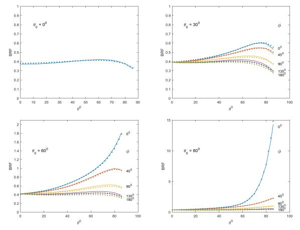
Figure 6. BRF of white ice at 885 nm, calculated with the RAY code (dots) and the asymptotic formula (curves).
