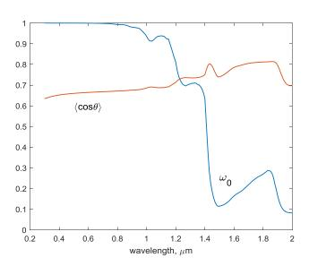
Figure 3. Spectral dependence of the photon survival probability and the average cosine for the random mixture 'ice-air' with the mean chord of 2 mm.
