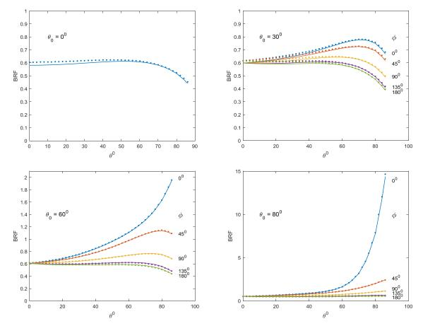
Figure 5. BRF of white ice at 490 nm, calculated with the RAY code (dots) and the asymptotic formula (curves).
