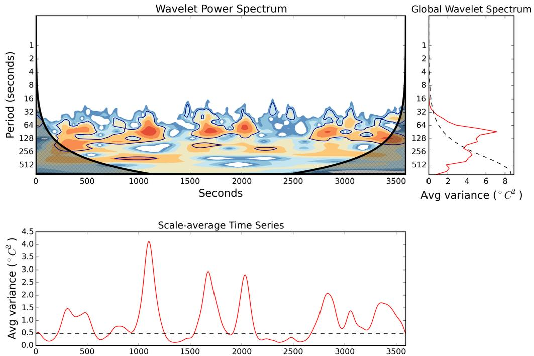
**Figure 7.** Example of a rectified wavelet power spectrum of the temperature signal at location Z2 for southerly flow (upper left column) , the time average-wavelet power spectra (right column), and the scaled-averaged time series (lower left column). Red and blue indicate high and low scaled powers (in base 2 logarithm), respectively. Black lines outline the wavelet spectrum at a 95% confidence level. The cross-hatched region marks the cone of influence, where edge effects become important.
