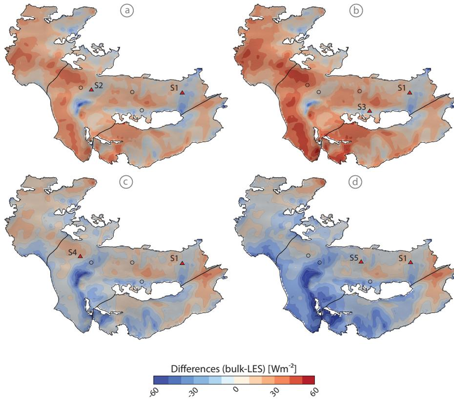
**Figure 11.** ~~Shown are the differences~~ Differences in the surface sensible heat fluxes between the LES and the bulk method. The cases A-D indicate different extrapolation scenarios based on the pseudo-observations ( $Z_0$  S1,  $Z_{a-a}$  S2-S5). Positive differences correspond to regions where the fluxes have been overestimated by the bulk approach.
