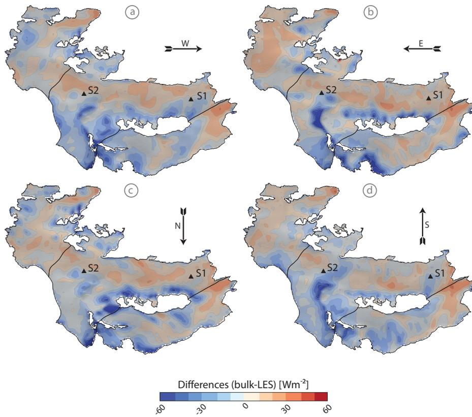
**Figure 10.** Differences in the mean surface sensible heat fluxes between the LES and the bulk method for different wind direction. Positive differences correspond to an overestimation of the surface heat flux by the bulk approach.
