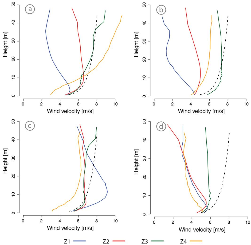
**Figure 5.** Vertical profiles of the mean wind velocity at the four sites (Z1, Z2, Z3 and Z4) for each case experiment. The dashed line represents a neutral logarithmic wind profile with  $z_0 = 0.01$  m and  $u_* = 0.3$   $\text{ms}^{-1}$ .
