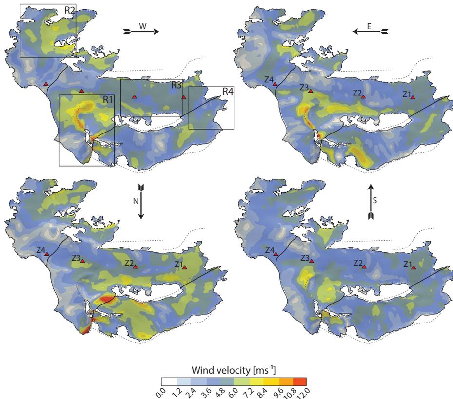
**Figure 3.** Mean velocity of the surface wind fields (2 m) for each of the four case experiment. The four boxes R1-4 and the sites Z1-4 define regions and locations on the glacier which are used for discussion in the results section. The grey dashed lines represent sharp ridges in the study area.
