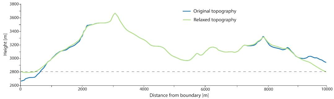
**Figure 2.** Adaption and relaxation of the computational domain. The blue and green lines show a east-west profile of the original and relaxed topography, respectively. The boundary grid cells have been set to the mean value of both cells (dashed line). The adjacent grid points are slowly relaxed (exponentially) to get a smooth transition from the boundaries towards the inner domain using a spline algorithm.
