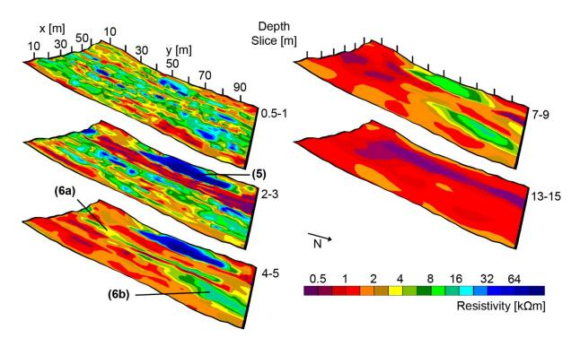
Fig. 6: Quasi-3D ERI Model Uertsch\_02. Numbers refer to structures described in the text. Chosen depth slices.
