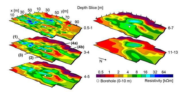
Fig. 5: Quasi-3D ERI Model Uertsch\_01. Numbers refer to structures described in the text. Chosen depth slices.
