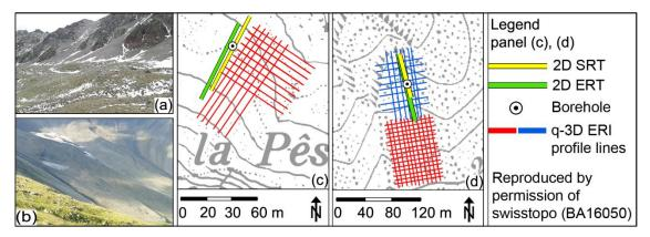
Fig. 1: Site overview and measurement setups. a) Photo Nair site b) Photo Uertsch site c) quasi-3D ERI setup Nair d) quasi-3D ERI setups Uertsch\_01 (blue lines) and Uertsch\_02 (red lines).
