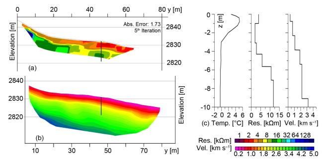
Fig. 2: Comparative analysis of (a) 2D ERT Profile, (b) 2D SRT Profile and (c) 1D Temperature/ Resistivity/ Velocity plots at Nair rockglacier.
