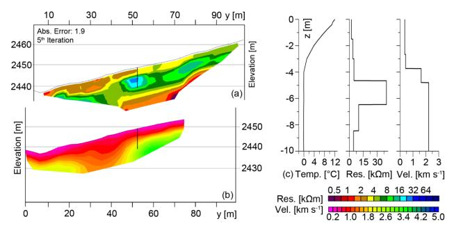
Fig. 3: Comparative analysis of (a) 2D ERT Profile, (b) 2D SRT Profile and (c) 1D Temperature/ Resistivity/ Velocity plots at Uertsch rockglacier.
