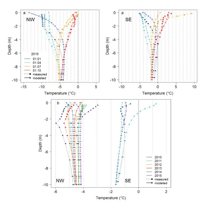
Figure 6. Evaluation of modelled bedrock temperature against measured bedrock temperature in the AdM NW and SE boreholes 5 at daily time-step (a) and annual time-step (b).
