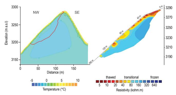
Figure 7. Model evaluation (left) against ERT transect (right) for October 2012 at the GM. The red line on the left figure 5 delineates the ERT contour.
