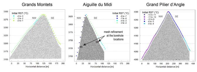
Figure 3: Boundary conditions: initial RST plotted over the models meshes for the three sites. The spatial resolution of the initial RST (coloured dots) has been refined at the mesh scale by linear interpolation. Below the topographies, a box of 5000 m elevation and a constant geothermal heat flux of 85 mW<sup>-2</sup> were set up.
