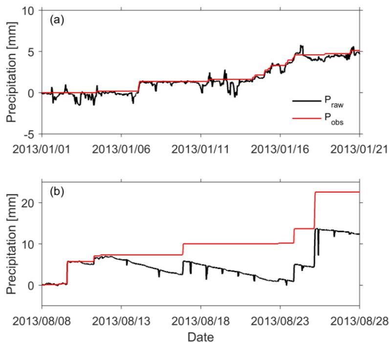
Figure 3 Examples of typical noise filtering for Geonor precipitation measurements ( $P_{raw}$ : raw data;  $P_{obs}$ : filtered data).
