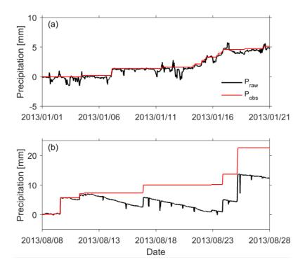
Figure 3 Examples of typical noise filtering for Geonor precipitation measurements ( $P_{raw}$ : raw data;  $P_{obs}$ : filtered data). (a) Diurnal drift, e.g. BC. (b) Evaporation caused drops, e.g. MC.
