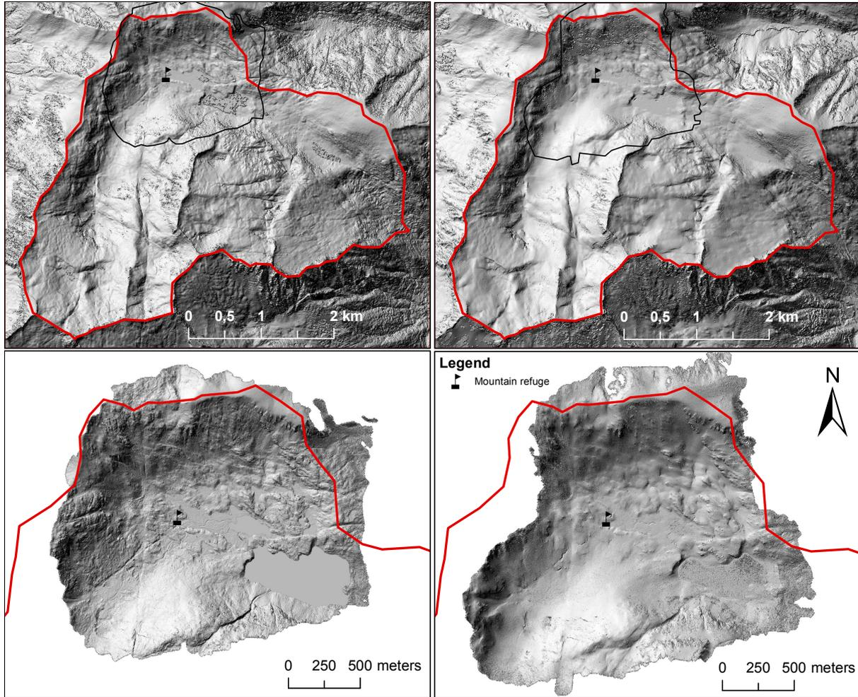
**Figure 5.** Hillshade of snow free 2 m-Pléiades (top-left) and 1 m-UAV DEM (bottom-left) DEMs, and winter 2 m-Pléiades (top-right) and 1 m-UAV (bottom-right) DEMs. The outlines of the UAV extents are indicated in the Pléiades extents.
