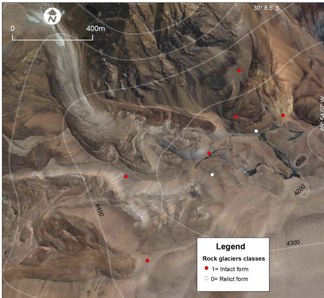
Supplementary figure 1: Examples of rock glaciers classified as intact (i.e. active or inactive) and relict on the southeast side of Cerro Tapado, Chile.
