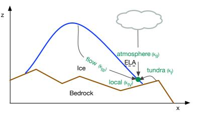
**Figure 2.** Cross section through an ice sheet: four different mechanisms of aerosol transport to the ablation zone. ELA stands for equilibrium line altitude.
