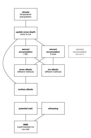
**Figure 3.** Flow chart of the surface mass balance model inside a loop which is solved for each time-step. Ultimately resulting in an annual SMB which can be used as boundary condition in an ice sheet model.
