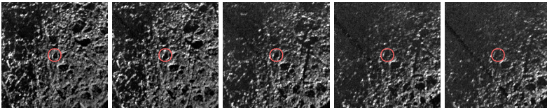
Figure 18. An example of manual VB pixel location estimation and VB location defined by the algorithm with a time step of 200 minutes (case A). The locations are shown in a: the red dots indicate the VB center location, the blue dots the selected and tracked feature location, the corresponding pairs have been marked with the green rectangles. The VB areas (red circles) in the radar imagery with some background included at the given time instants are shown in time order from left to right in b-f.
