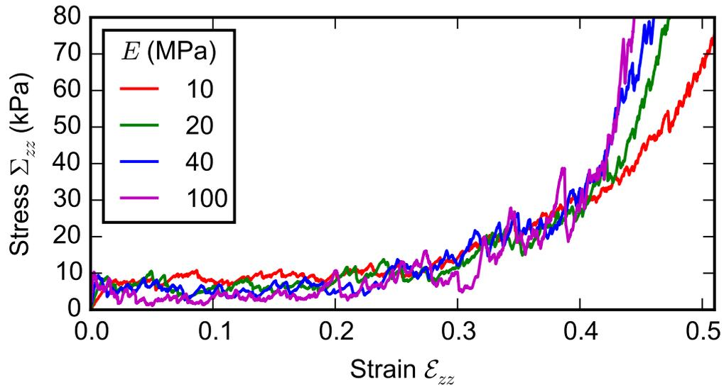
**Fig. 2.** Computed stress-strain curves for different Young's moduli.
