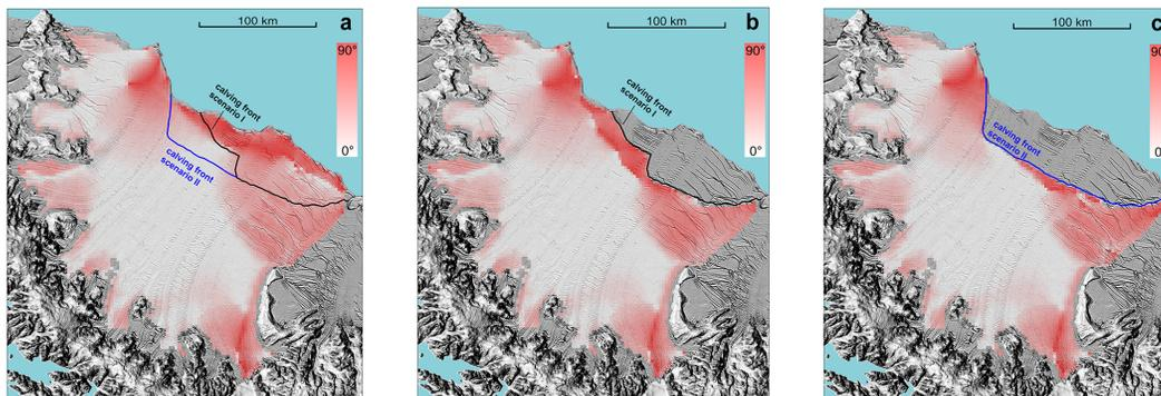
**Figure 3.** Results from ice shelf flow model: Stress-flow angle fields for the present day ice front geometry (a) and for the new geometries under Scenarios I (b) and II (c).
