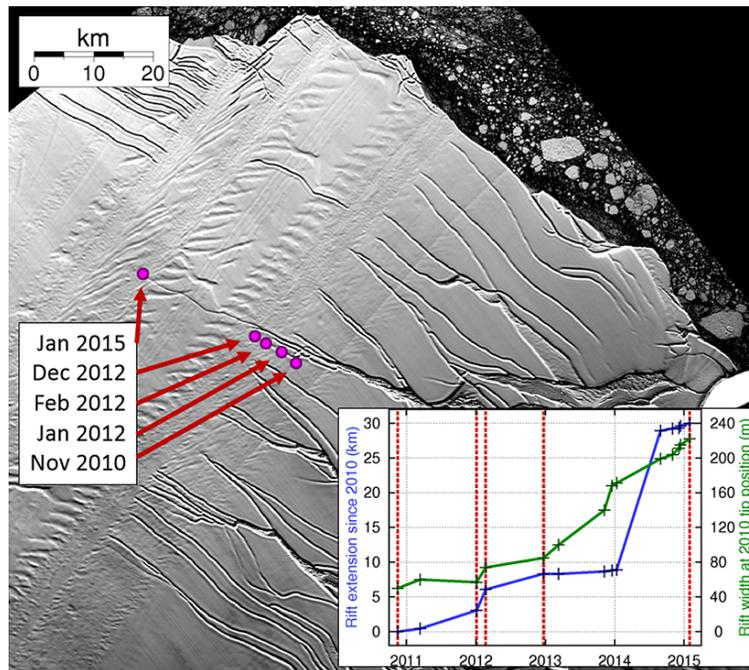
**Figure 2.** Analysis of rift propagation using Landsat data. Background image, in which the rift is visible, is from 4 December 2014. Inset graph shows the development of rift length with respect to the 2010 tip position, and rift width at the 2010 tip position, measured from 15 Landsat images (crosses). Circles and labels on the map, and dotted red lines on the graph, show the positions of notable stages of rift development.
