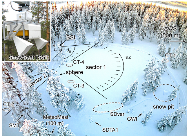
Figure 5. The radar data and meteorological measurements were acquired on the above shown test site nearby the town of Sodankylä, Finland. The SnowScat Instrument SSI (inset) was mounted on a 9 m high tower. The reference target (sphere) used for calibration can be located behind a tree. The SSI scanned sector 1 and 2 with different azimuth ( az ) and incidence angles \theta_0 . The meteorological sensors SMT, MétéoMast, SDAT1, GWI, and AWS are specified in Table 1. Snow profiles were taken at CT-1 to CT-4 for analysis by computer tomography. Snow density was measured in the snow pit, with the Gamma water Instrument (GWI), and was also derived from the snow water equivalent (SWE) determined by the SSI as described in Leinss et al. (2015). The variability of snow depth was measured with seven sticks inside the ellipse "SDvar".
