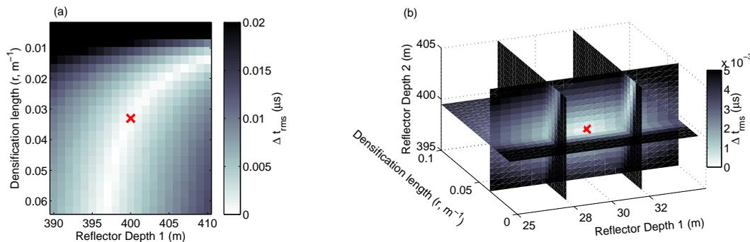
**Figure 4.** Traveltime residuals ( $\Delta t_{rms}$ ) calculated with raytracing between ideal reflector in a fixed depth–density profile ( $A = 460 \text{ kg m}^{-3}$ ;  $r = 0.033 \text{ m}^{-1}$ ) with reflectors perturbed in terms of depths and density. Ideal solutions are marked with red crosses: **(a)** traveltime residuals for an ideal reflector at 400 m depth; **(b)** volumetric slice plot of traveltime residuals for two idealised reflectors at 30 and 400 m depth.
