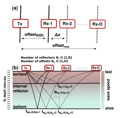
**Figure 1. (a)** Plain view of the wide-angle acquisition geometry: Transmitting (Tx) and receiving (Rx) antennas were aligned in parallel. While the transmitter remained at a fixed location, the receiver was incrementally moved farther away. A sketch of the corresponding raypaths is shown in **(b)** with a synthetic velocity—depth function color coded. The labels of example rays and their incidence angles are presented in Eqs. (1)–(10).
