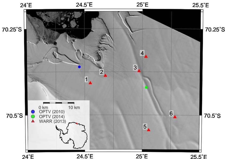
**Figure 2.** Location of the wide-angle (WARR) radar sites (red triangles) relative to the boreholes of 2010 and 2014 which were used for optical televiewing (OPTV). The depressed surfaces of ice-shelf channels appear as elongated lineations in the background image (Landsat 8, December 2013 provided by the US Geological Survey).
