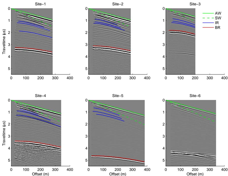
**Figure 3.** Wide-angle radar data showing air waves (AW, green lines) and surface waves (SW, green dashed lines) with linearly increasing traveltime with offset, while traveltime increases hyperbolically with offset for internal (blue) and basal (red) reflectors. See Fig. 2 for locations of Sites 1–6. Site 6 was excluded from further analysis because the basal reflection is ambiguous (probably due to off-angle reflectors in the vicinity).
