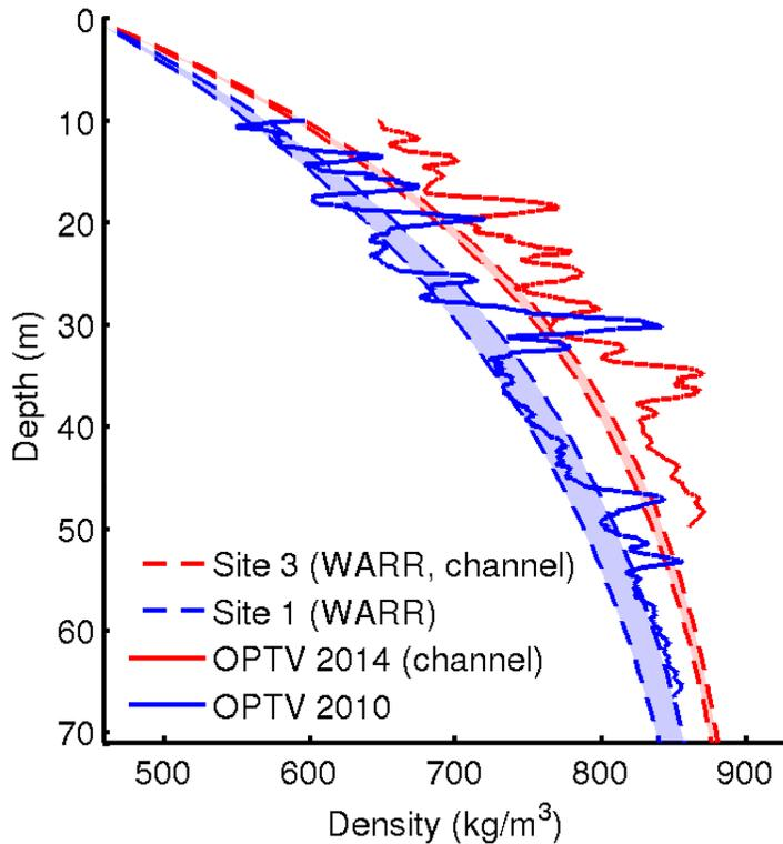
**Figure 7.** Depth profiles of density derived from WARR (dashed) and OPTV (solid). WARR data are from Sites 1 and 3, closest to the OPTV sites. Site 3 and the 2014 borehole are both in the trough of an ice-shelf channel (Fig. 2). The envelopes of the radar-derived densities correspond to the lower and upper limit of five reflector combinations used for the inversion. The OPTV logs were smoothed with a 0.5 m running mean.
