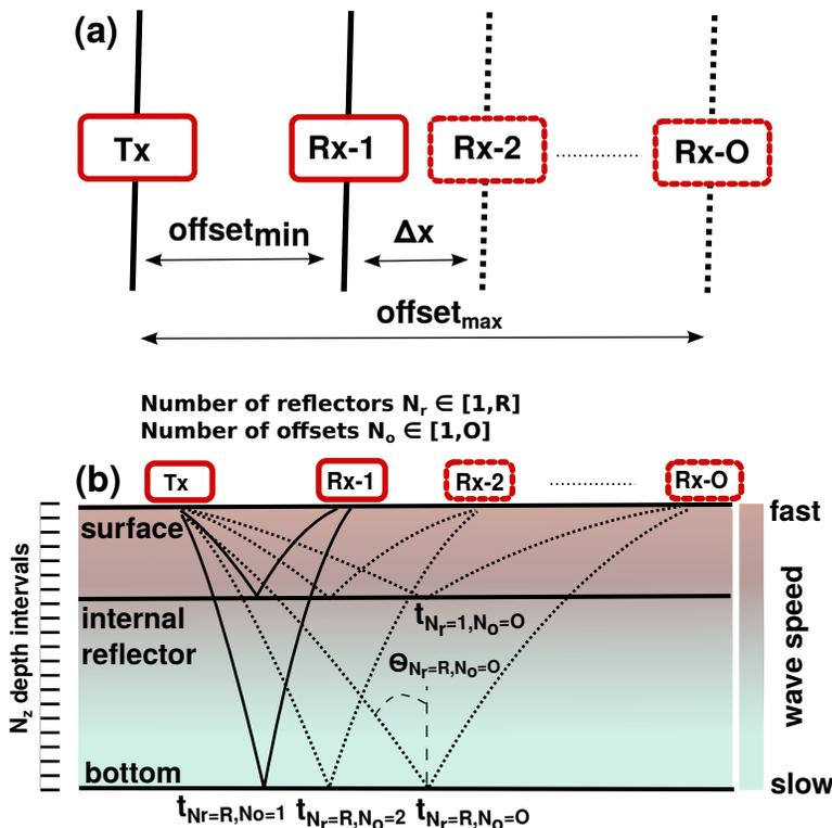
**Figure 1.** (a) Plain view of the wide-angle acquisition geometry: Transmitting (Tx) and receiving (Rx) antennas were aligned in parallel. While the transmitter remained at a fixed location, the receiver was incrementally moved farther away. A sketch of the corresponding raypaths is shown in (b) with a synthetic velocity–depth function color coded. The labels of example rays and their incidence angles are presented in Eqs. (1)–(10).
