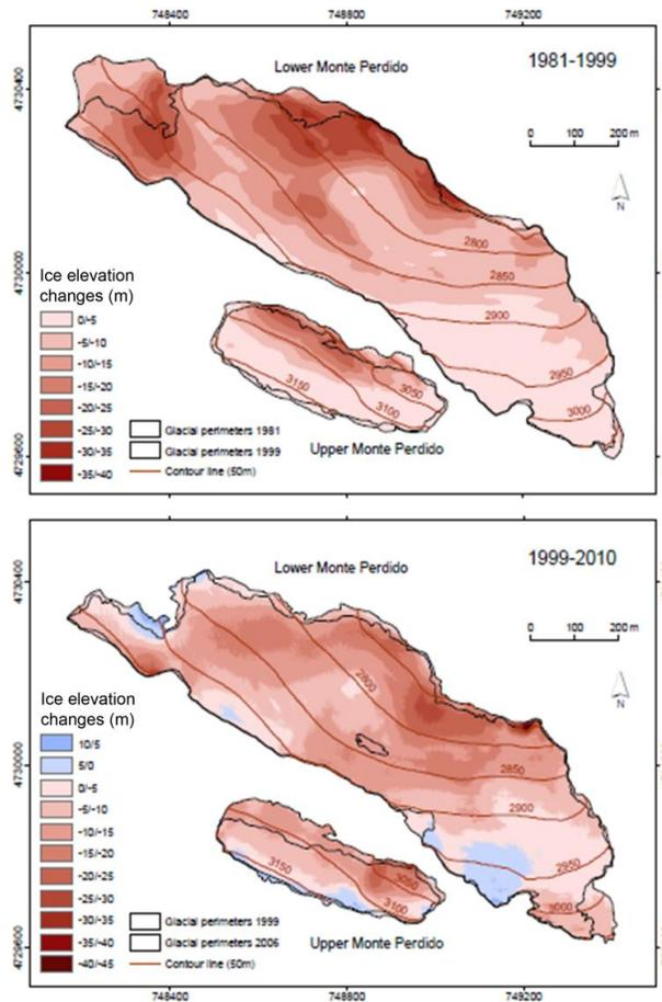
**Figure 4.** Changes in ice thickness in the upper and lower Monte Perdido Glacier from 1981 to 1999 and from 1999 to 2010 based on comparison of DEMs.
