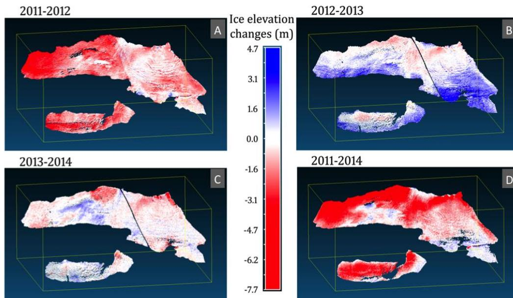
**Figure 5.** Changes in ice thickness based on terrestrial laser scanning from September of 2011 to 2012 (a), 2012 to 2013 (b), 2013 to 2014 (c), and 2011 to 2014 (d).
