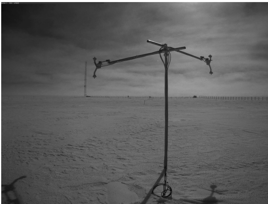
Figure 1. Spectral albedo measurement at Dome C (picture taken on 12 January 2014, 11:00 local time ). The vertical mat-mast is approximately 2.22 m high.
