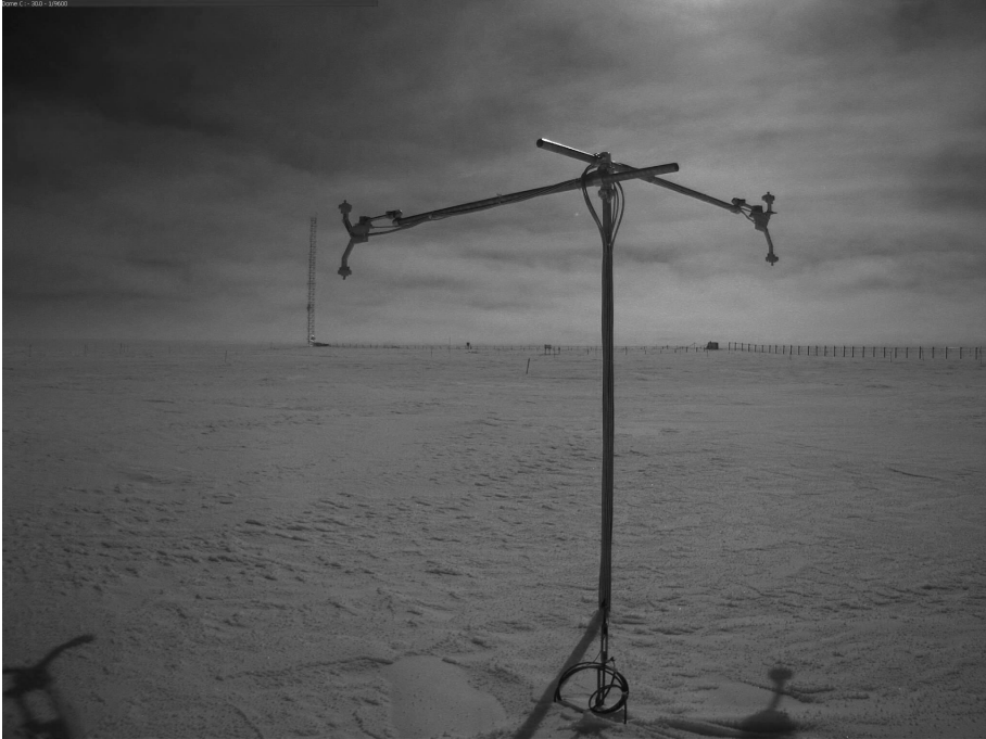
Figure 1. Spectral albedo measurement at Dome C (picture taken on 12 January 2014, 11:00 local time). The vertical mast is approximately 2 m high.
