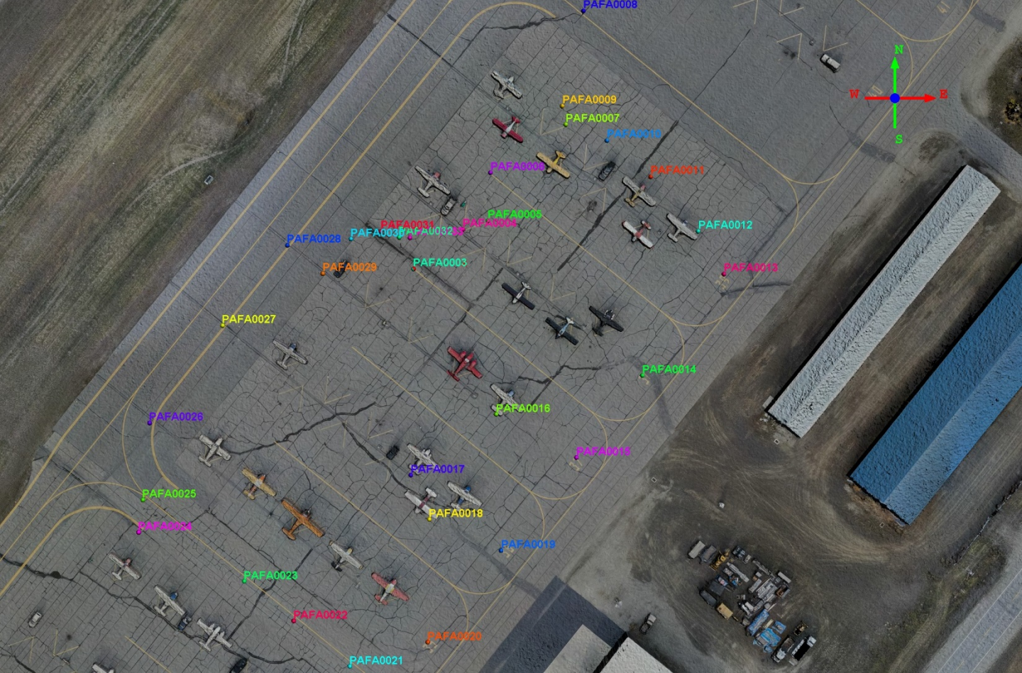
Figure SOM2 A-B. GCPs from Fairbanks International Airport. These photo-identifiable GCPs were made on taxiways letter and intersections of lines or cracks.
