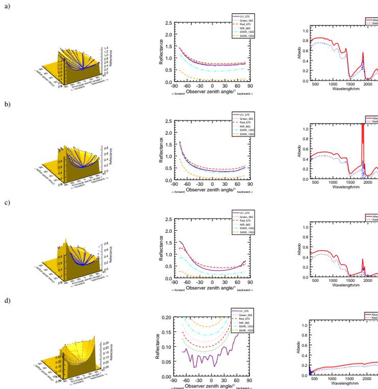
**Figure 11.** As in Fig. 9. **(a)** 10 mL of silt /  $0.5 \text{ m}^2$  on top of snow, on the 4 April 2013 at 15:05,  $65^\circ$ , **(b)** 10 mL of silt /  $0.5 \text{ m}^2$ , on the 4 April 2013 at 16:29,  $72^\circ$ , note large SZA, **(c)** same sample on the 5 April 2013 at 11:16,  $61^\circ$ , most difference to b due to different SZA, **(d)** pure silt measured in laboratory,  $65^\circ$ .
