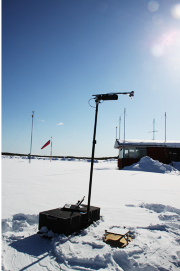
Figure 2. FIGIFIGO at the SoS test site at the Sodankylä airport. A clean snow sample has been measured, and the last reference measurement with the white Spectralon panel is being taken. Deep and soft snow complicated the usability of FIGIFIGO. While the movements in the snow left significant traces, the target area under the instrument footprint was carefully kept untouched during the measurement.
