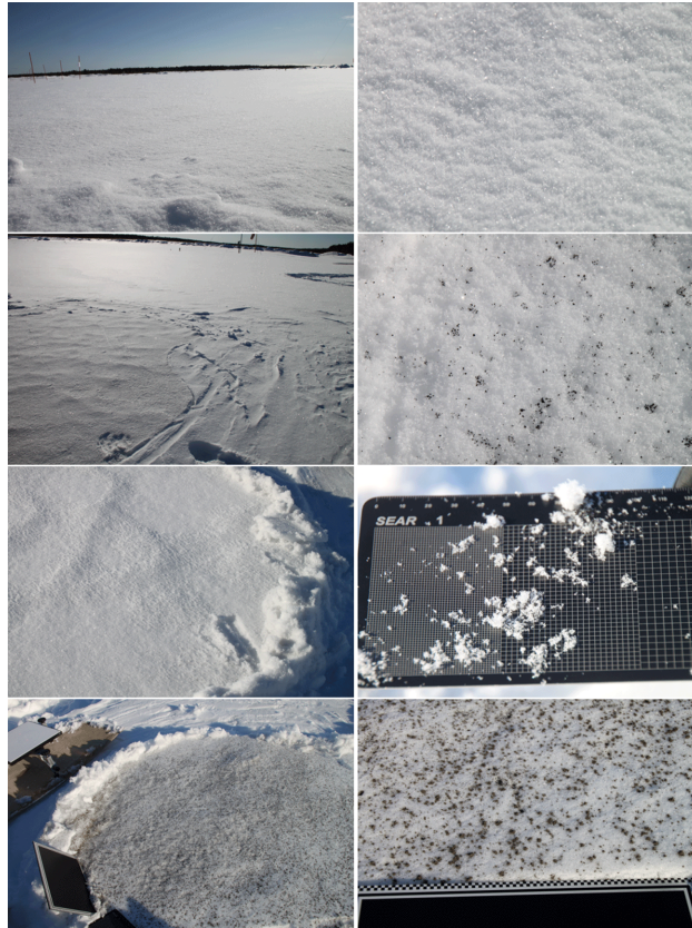
Figure 3. Photographs of the samples. Left an overview, right some details. From the top, clean snow 4 April 2013, snow deposited with volcanic ash 3 April 2013, snow deposited with chimney soot 4 April 2013, and on the bottom snow deposited with glaciogenic silt 4 April 2013.
