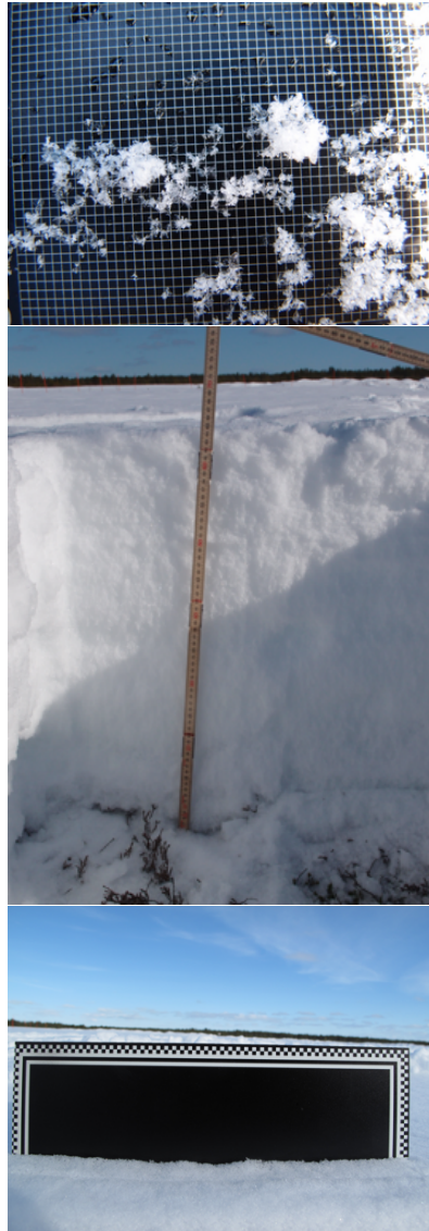
Figure 4. More snow profiles taken on the 3 April of unprocessed snow near the FIGIFIGO spot. Because of near zero temperature, the snow crystals melt fast on the black plate, and the smallest details and grains have already disappeared.
