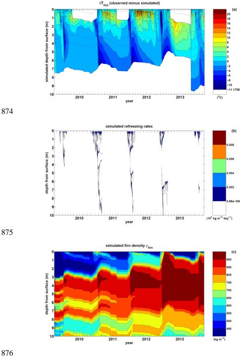
Figure 11. (a) Difference between firn temperature measured by the KAN\_U thermistor string and simulated firn temperature. The blue lines indicate the position of the thermistors below the surface. The white areas near the surface are due to surfaced thermistors. Note that the thermistor string was replaced by a new one drilled on 28 April 2013. (b) Simulated refreezing rates. (c) Simulated firn density.
