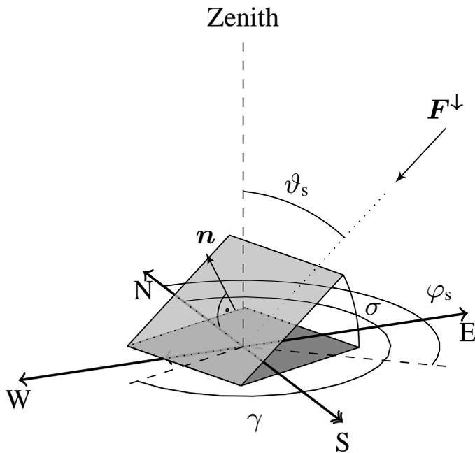
**Figure 2.** Geometric account of a tilted surface.
