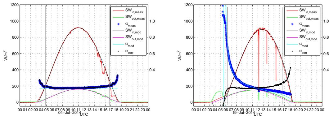
**Figure 7.** Measured, modeled and corrected  $SW_{in}$ ,  $SW_{out}$  and  $\alpha$  with a horizontally levelled (left) and an intentionally inclined pyranometer (right) at WHW for two days in July 2014.
