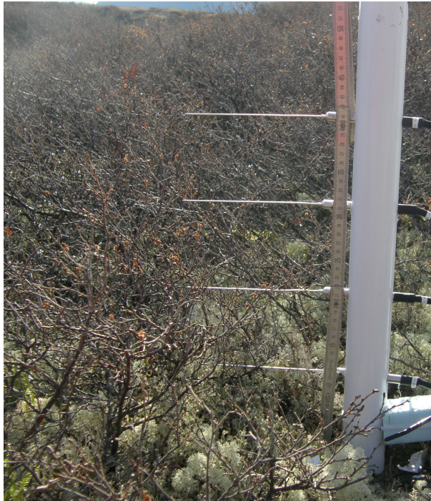
Figure 1. Photograph of the four TP02 needle probes deployed in shrub tundra. The photo was taken on 6 October 2014, when the dwarf birch had grown to about 30 cm high.
