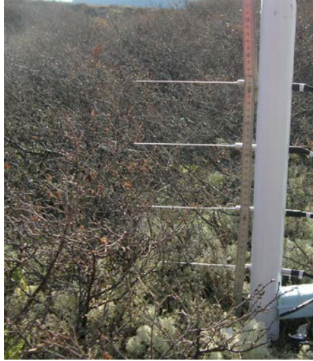
Figure 1. Photograph of the four TP02 needle probes deployed in shrub tundra. The photo was taken on 6 October 2014, when the dwarf birch had grown to about 30 cm high. The needle probes are 14, 24, 34 and 44 cm above the ground-lichen interface.
