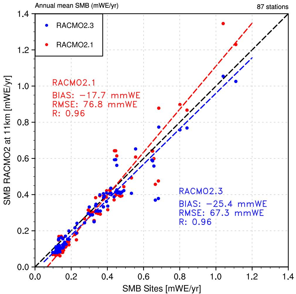
**Fig. 8.** Observed and simulated SMB (mWE/yr) across the accumulation zone of the GrIS averaged for the period 1979–2012. The regression lines are displayed as dashed lines for RACMO2.3 (blue) and 2.1 (red). For observation locations, see yellow dots in Fig. 1.
