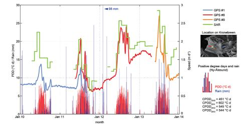
**Figure 6.** Time series of speed of Kronebreen between 2010 and 2013 linked to water supply by melt (positive degree days (°C) and rain events (mm) from weather station in Ny-Ålesund). Speed of Kronebreen (md<sup>-1</sup>) derived from RS-2 (green) and GPS (blue/red/orange).
