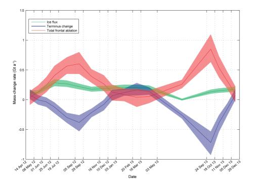
**Figure 8.** Frontal ablation of Kronebreen between 14 April 2012 and 29 December 2013 and components, ice flux and terminus position changes. Note that the ice flux could not be estimated between May and September 2013 and therefore set to 0.0 Gta<sup>-1</sup> as the quality of the speed map was not sufficient to extract glacier speed along the fluxgate.
