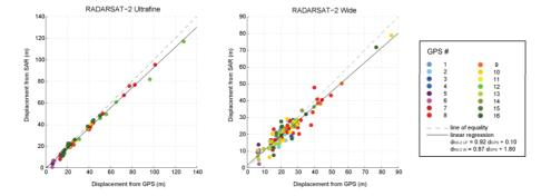
**Figure 3.** Validation of glacier displacement: displacements extracted from SAR maps at the position of GPSs and plotted against GPS displacements **(a)** RS-2 UF vs. GPS **(b)** RS-2 W vs. GPS.
