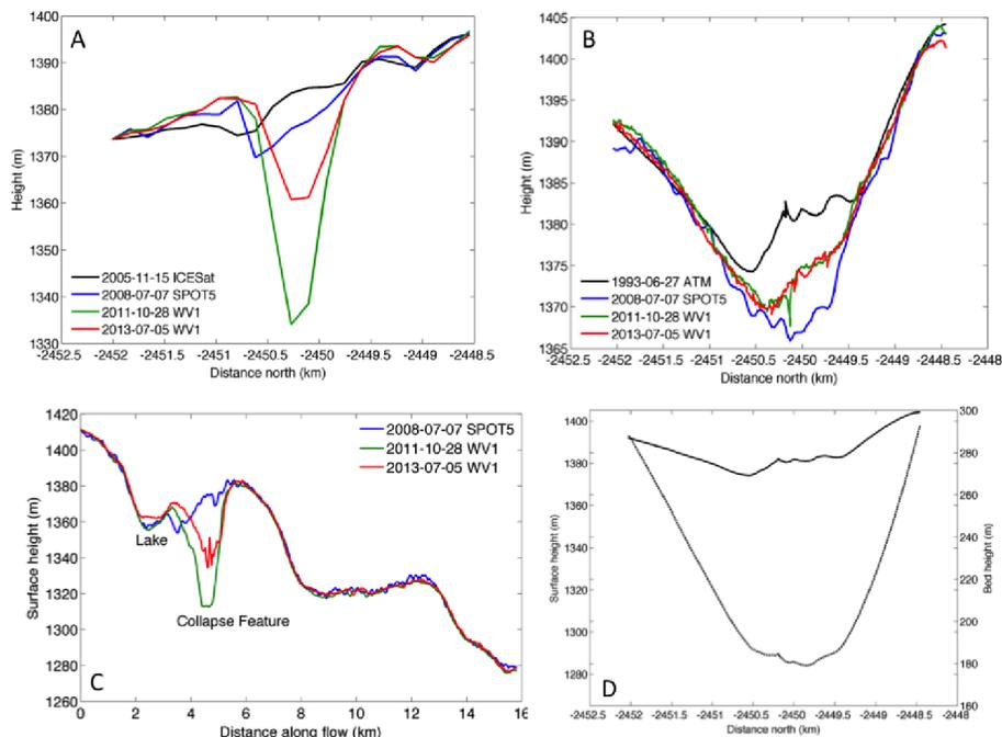
**Figure 3.** Surface elevations from laser altimetry and stereoscopic Digital Elevation Models (DEM's) along the (a) 15 November 2005 ICESat-1 and (b) 26 June 1993 ATM tracks shown in Fig. 2. (c) Along-flow (east to west) surface elevation profiles through the center of the depression from three stereoscopic DEM's. (d) (solid curve) Surface and (stipples) bed heights for the 1993 airborne survey over the eastern portion of the depression (see Fig. 2). Both vertical axes have the same scale.
