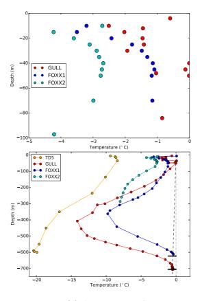
**Figure 2.** Measured ice temperatures. **(a)** shows near-surface temperatures at sites GULL and FOXX. Holes FOXX1 and FOXX2 are 86 m apart. **(b)** shows measured ice temperatures in four boreholes at the drill sites TD5 (Swiss Camp; data from Thomsen et al., 1991), GULL and FOXX. The dashed line indicates the pressure melting temperature.
