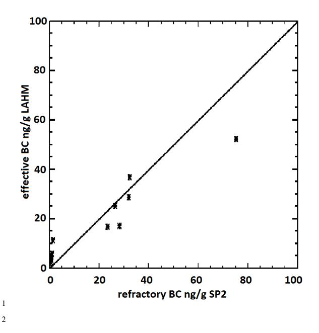
Figure 5. Plot showing the relationship between eBC as determined from the LAHM analysis and refractory black carbon as determined by the SP2 instrument ( $r^2=0.92$ ). The values near 0.0 refractory BC are from Pisco mountain in region 2 while the higher values are from Vallunaraju in region 4. The 1 to 1 line is plotted to guide the eye.
