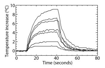
Figure 2. Measured temperature profiles for 7 filters with a variety of light absorbing particle loads. Temperature recording started ten seconds before the lamp was illuminated, and the lamp was extinguished 30 seconds later. Temperatures are normalized to the average of first 10 seconds of data and the temperature usually returned to the start temperature within a minute of the lamp being extinguished.
