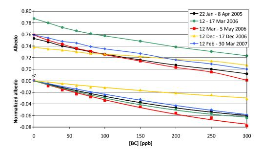
Figure 6. (Top) Simulated average albedo for several periods with continuous snow higher than 10 cm as a function of BC concentration. (Bottom) Normalized albedo as differences of the averaged albedo minus the averaged albedo at BC = 0. The lines correspond to the best fit of a quadratic polynomial forced through zero for each set of the normalized albedo.
