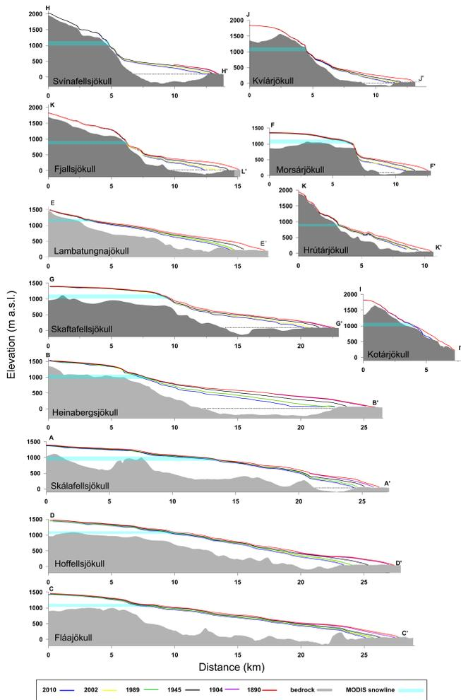
**Figure 7.** Longitudinal profiles of the southeast outlet glaciers, showing ice thickness and location of the termini at different times. The average ELA derived from the MODIS images is shown with a light blue horizontal line. Öræfajökull outlets with dark gray colored bedrock basal topography and the eastern outlets with light gray colored bedrock basal topography.
