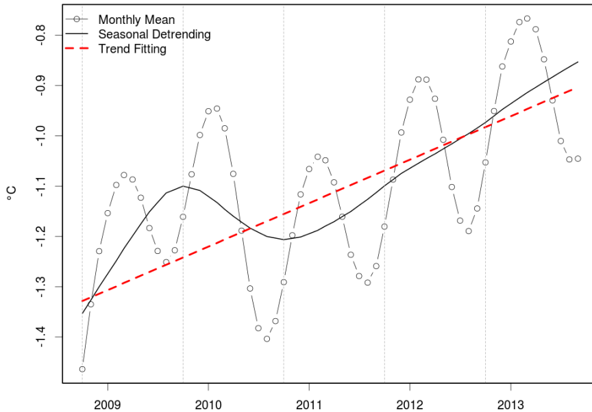
Figure 3. Methodological steps of trend analysis: (1) monthly aggregation, (2) seasonal detrending, (3) trend fitting. Vertical dashed lines represents the 1 October, materializing the limits of the hydrological years.
