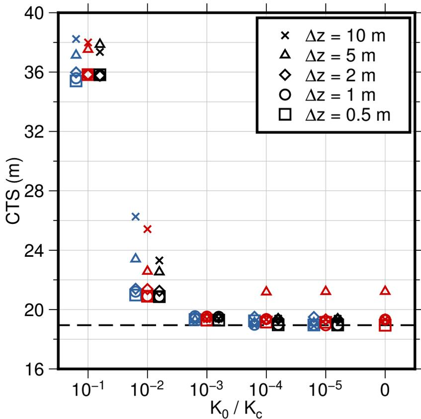
**Figure 3.** Comparison of simulated steady state CTS positions for different values of the temperate ice conductivity in Experiment B. The different models are shown as: TIM-FD<sup>3</sup> (blue), ISSM (red) and COMIce (black). Results of different models are slightly shifted on the  $x$  axis to not overlay each other. The dashed black line indicates the CTS position of the analytical solution derived for  $K_0 = 0$ .
