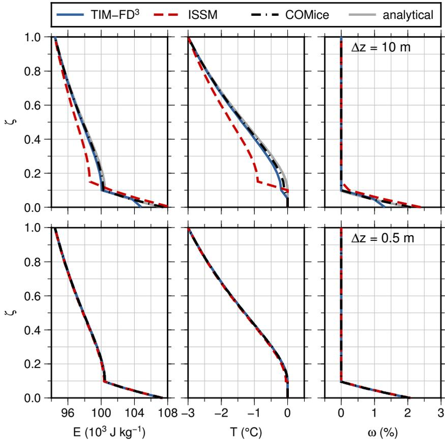
**Figure 4.** Simulated steady state profiles of the enthalpy,  $E$ , the temperature,  $T$ , and the water content,  $\omega$  for TIM-FD<sup>3</sup> (blue), ISSM (red) and COMice (black) compared to the analytical solution (gray).  $\zeta = z/H$  is the normalised vertical coordinate. The vertical resolution is  $\Delta z = 10$  m (upper row) and  $\Delta z = 0.5$  m (lower row),  $CR = K_0/K_c = 10^{-5}$ . In the lower row the model results overlay the analytical solution.
