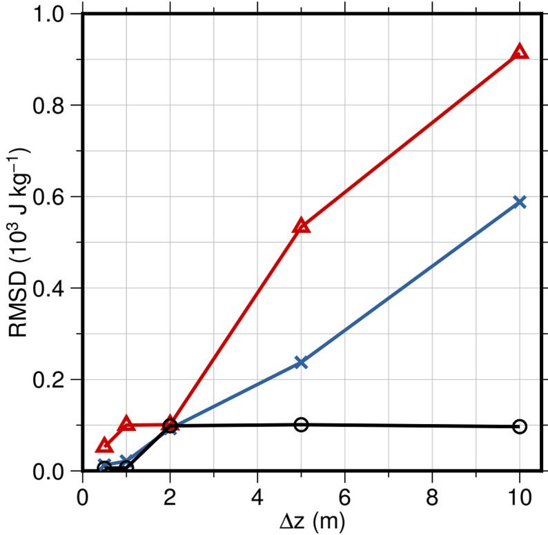
**Figure 5.** The root-mean-square deviation (RMSD) of the model results to the analytical solution (Experiment B) for different vertical grid resolutions  $\Delta z$ . Model results for TIM-FD<sup>3</sup> (blue crosses), ISSM (red triangles) and COMIce (black circles) are obtained for the lowest conductivity ratio  $CR = K_0/K_c = 10^{-5}$  applied to all models.
