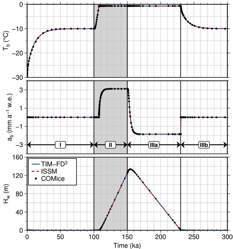
**Figure 1.** Results for Experiment A simulated with TIM-FD<sup>3</sup> (blue), ISSM (red) and COMice (black) overlay each other. Phases I to III are described in the main text. The warming phase II is shaded in grey.
