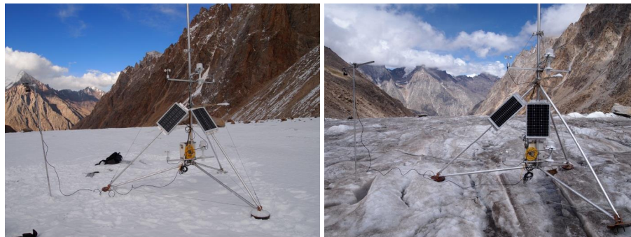
Figure 2. Photographs of AWS1 on Chhota Shigri Glacier taken on 09 October 2012 (left panel) and on 22 August 2013 (right panel) (©: Mohd. Farooq Azam). SR50A mounted on a separated pole drilled into the ice, is visible at the left of AWS1.
