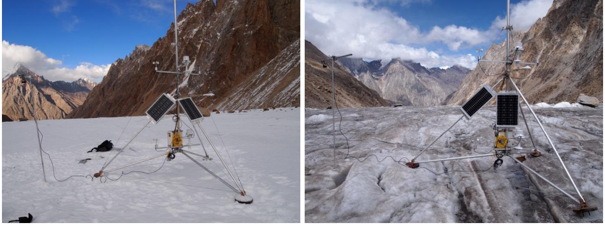
Fig. 3. Photographs of AWS1 on Chhota Shigri Glacier taken on 09 October 2012 (left panel) and on 22 August 2013 (right panel) (©: Mohd. Farooq Azam). SR50A mounted on a separate pole drilled into the ice, is visible to the left of AWS1.
