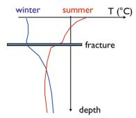
**Example Figure:** if temperature gradient is similar on both sides of fracture no heat sink (summer); if inflection to left fracture acts as heat sink (winter). Location of thermistors relative to the fracture is important!
