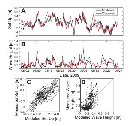
Fig. 10. Measured and modeled set up and wave height for summer 2009. Buoy was deployed in 2.2 m water depth.
