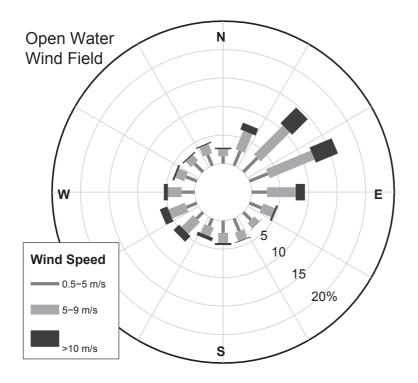
Fig. 3. Wind field at Drew Point during both the sea ice (A) and the sea-ice-free season (B). The wind field is dominated by wind from the ENE but show a smaller secondary maximum from the WSW (data from Urban and Clow, 2013).
